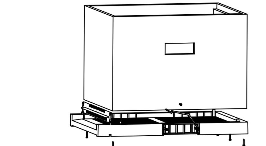
FIXER LE FOND AVEC DES VIS Art.V08 OU AVEC UN CROCHET A RESSORT Art.G02
